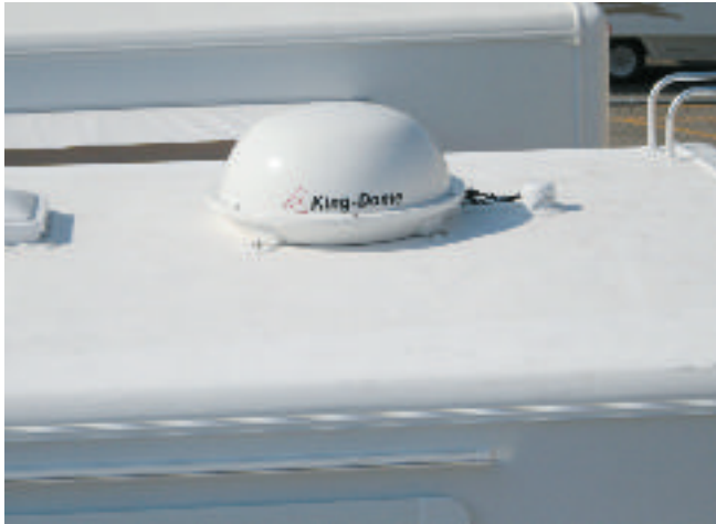
In-Motion Tracking Roof Mounted Satellite Dish with Dual LNB - finds the satellite automatically, even when the coach is in motion!
