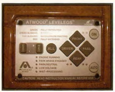
Four Point Fully Automatic Leveling System
