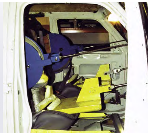
These 2 photos depict simultaneous seat belt pull testing and seating system testing. Seat belt testing confirms proper seat belt location and minimizes the possibility of anchorage failures. Seating system testing verifies the integrity of the seats, their attachments, mounting hardware and installation.
