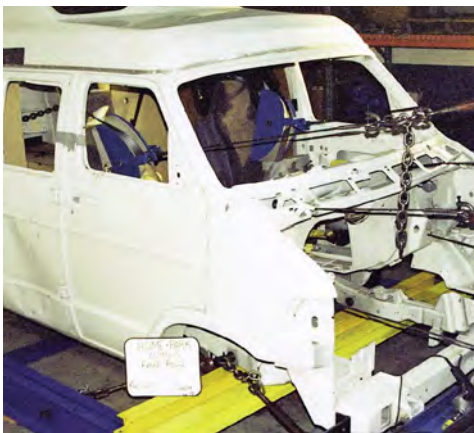
These 2 photos depict simultaneous seat belt pull testing and seating system testing. Seat belt testing confirms proper seat belt location and minimizes the possibility of anchorage failures. Seating system testing verifies the integrity of the seats, their attachments, mounting hardware and installation.
