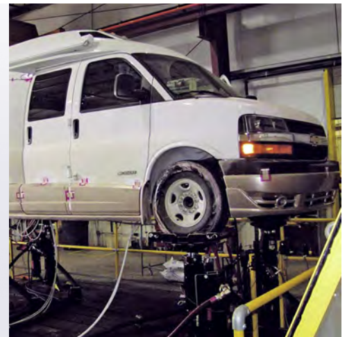
“Automotive manufacturer” style durability testing allowed us to quickly identify and implement numerous design improvements which would otherwise only become apparent during the normal life of the first ones of each new model built and sold.
